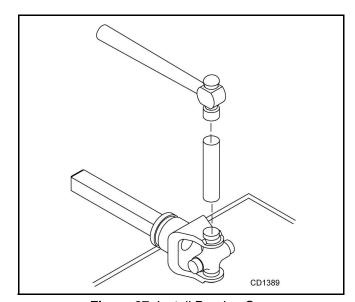
Figure 27. Install Bearing Cups
